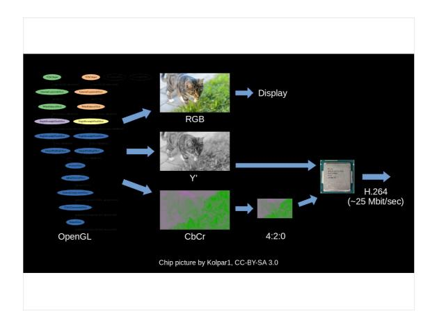
There's one detail we haven't talked about here yet, namely output. Uncompressed 720p60 video (4:2:0) is almost 700 Mbit/sec, or 300 GB/hour. This is possible to stream on a LAN, but very inconvenient to store. And we're actually quite out of CPU, so any codec we employed would have to be cheap.
