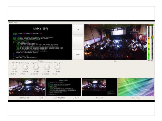
All the compressors have been working on objective values, but we want the final level to be around 0 LU on the R128 scale. So we have a final makeup gain that continuously reads the R128 meters and tries to adjust the gain very slowly to end up in the right place.
