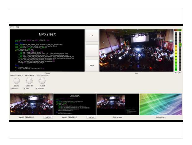
Now comes the real compressor, with typical voice settings (5 ms attack, 40 ms release). It has the effect of making the voice sound a bit tighter, more level and just overall better.
