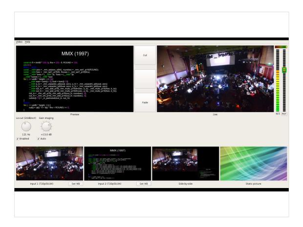
Then, we have what's essentially a very slow compressor (500ms attack, 20 seconds release). This is set so that the overall sound level is about right; or actually, a bit over the correct point.
