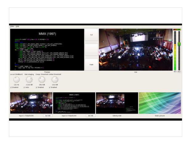
The third and final compressor in the chain is a limiter, basically a compressor with very high ratio. It's there as an emergency brake for really loud transients that got through the other compressors. Have you ever had your ears blown out by a presenter suddenly coughing into the mic? That is why you want a limiter.
